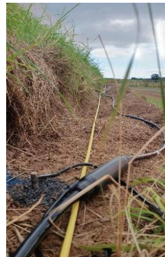
Figure 2: PRIME cable showing the electrodes through which a current is injected into the embankment. There are 512 electrodes in the Powderham Banks system.
