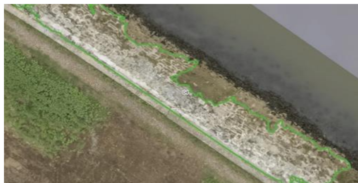
Figure 6: An example of a marine mortar repair (estuary face) and excavation and re-compaction repair to a piping failure (landward face). The marine mortar repair costs ~£100k less for the extents shown
