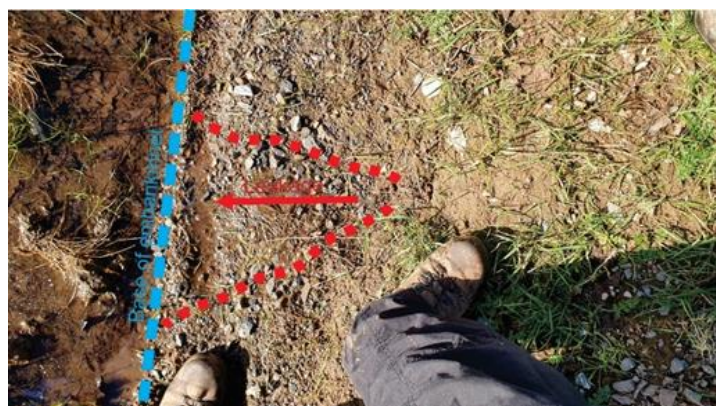
Figure 5: Low-level leakage identified at the location of 'January resistivity south' from the PRIME data.
