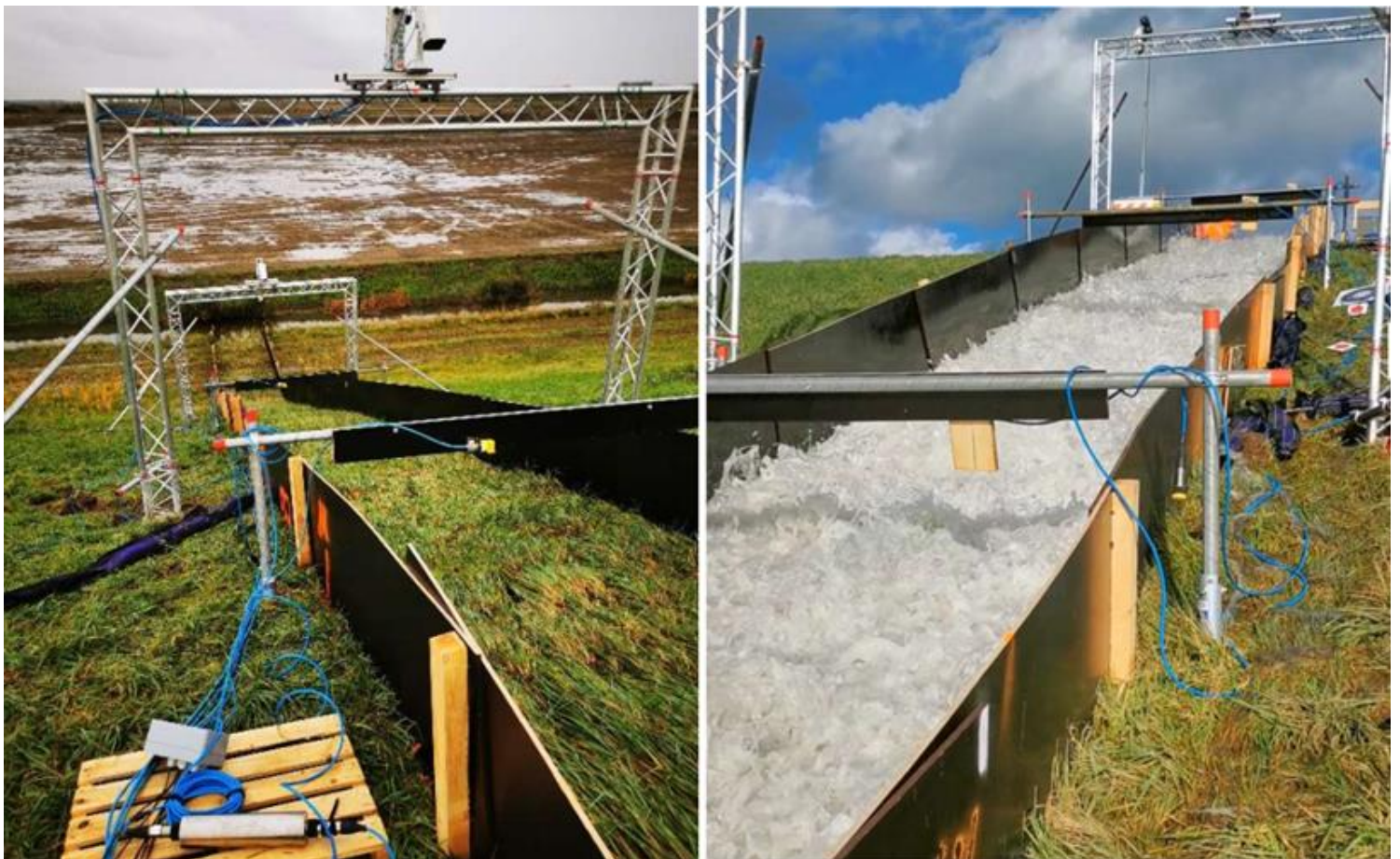
Figure 1: View of the setup and monitoring system on the levee slope before and during overflow. The installation features overhead cameras, and water level and velocity meters.
