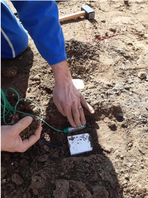
Volumetric water content and suction probes in La Riche's levee (France) (Source : Yasmina Boussafir, UGE)
