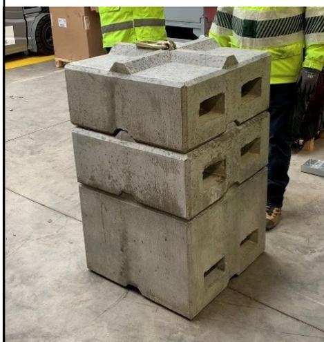
Low carbon concrete blocks of 250kg or 500kg mass.
