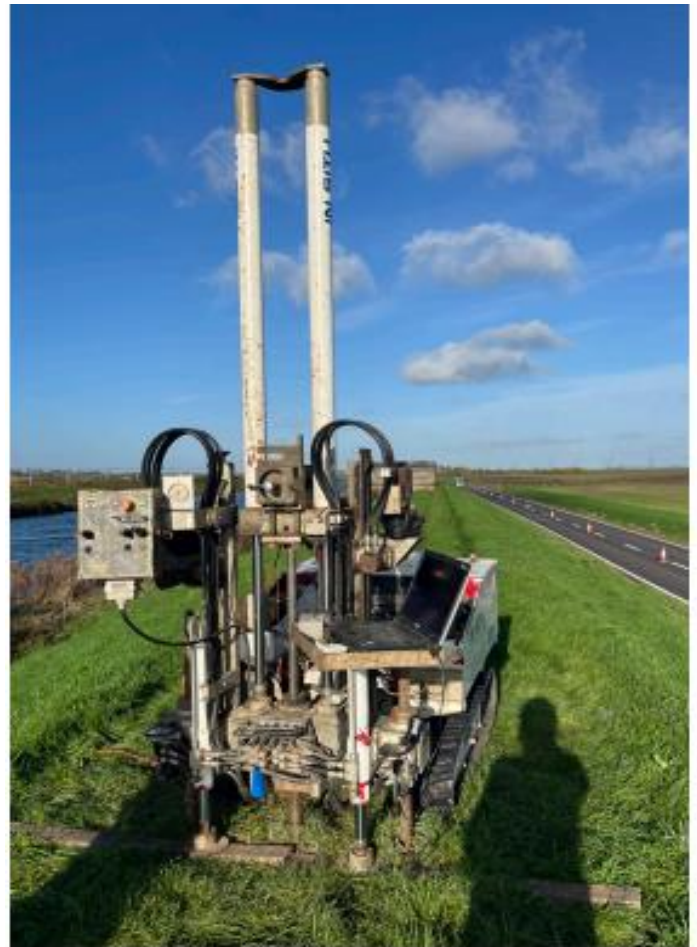
Figure 1: Cone Penetration Testing (credit: Georgie-Lee Heele)
