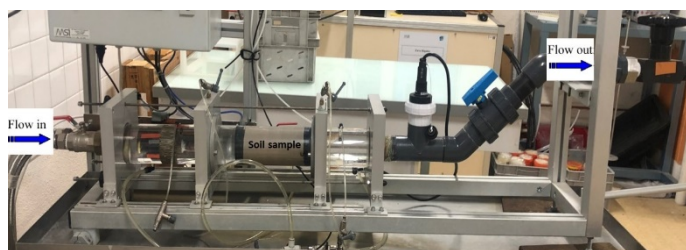
Figure 2: photograph of the INRAE's hole erosion test apparatus (HET)
