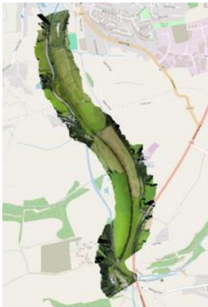
Figure 5: Georeferenced machine vision outputs converted into spatial polygons suitable for GIS analysis.
