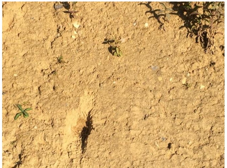
Figure 1: Photos taken in 2014 on the experimental embankment in Rouen: attempts to dig burrows in 2.5% lime-treated silt (photos D. Puiatti)
