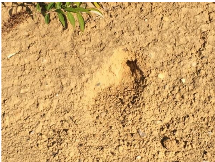
Figure 1: Photos taken in 2014 on the experimental embankment in Rouen: attempts to dig burrows in 2.5% lime-treated silt (photos D. Puiatti)
