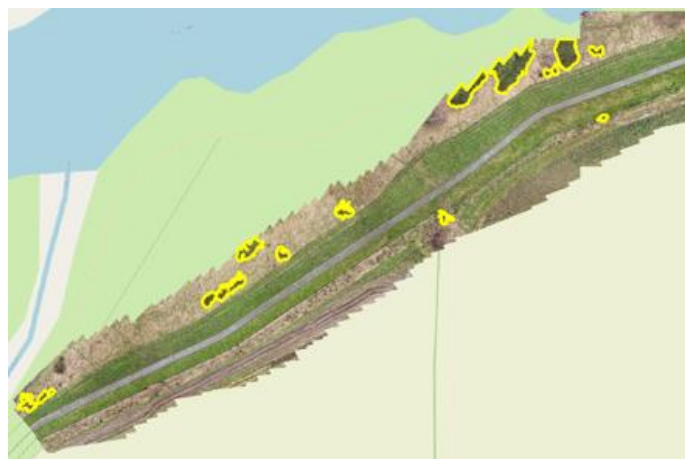
Figure 1: Example of machine vision identifying potential surface features from UAV survey imagery
