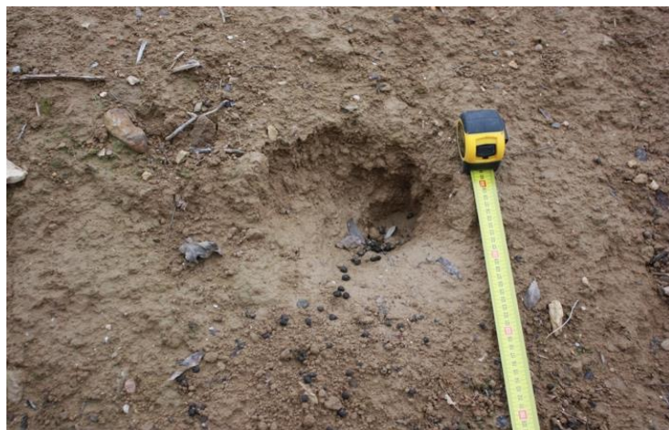
Figure 4: Attempts to dig burrows in the treated part of the dike (photo DigueELITE)
