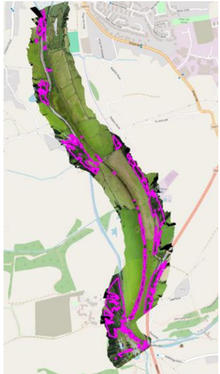
Figure 4: Example of detected features represented as mapped polygons on a surveyed flood Defence asset
