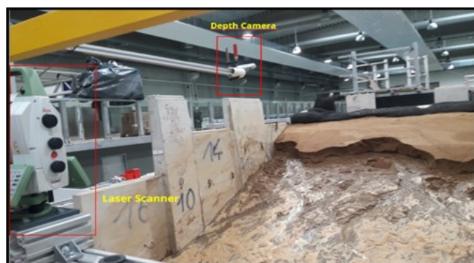
Figure 2: Monitoring of the landward slope during the failure of scenario GS02 by laser scan and depth camera
