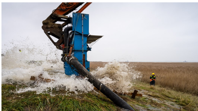
Figure 12: Wave impact generator in action. Photograph from Mischa Keijser
