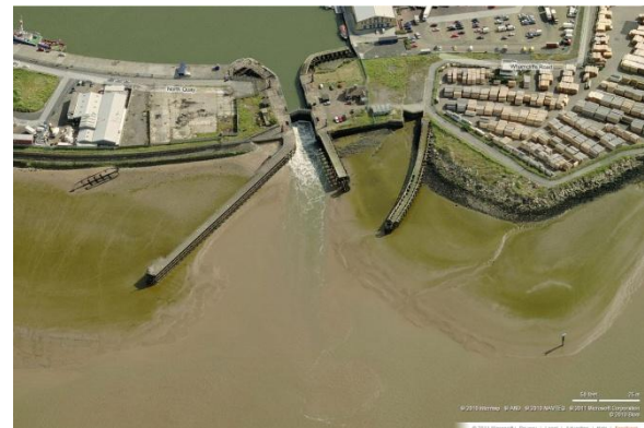
Photo 5.3 Complex mixture of levees, cutoffs, jetties and locks (Humber Estuary, UK)
